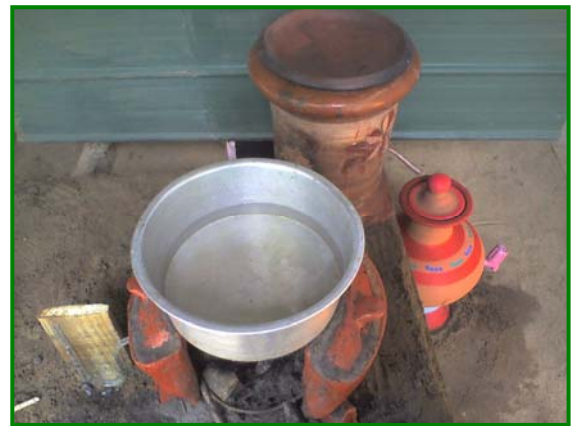
Figure 06: Firewood hearth distiller Front view and field experiment
